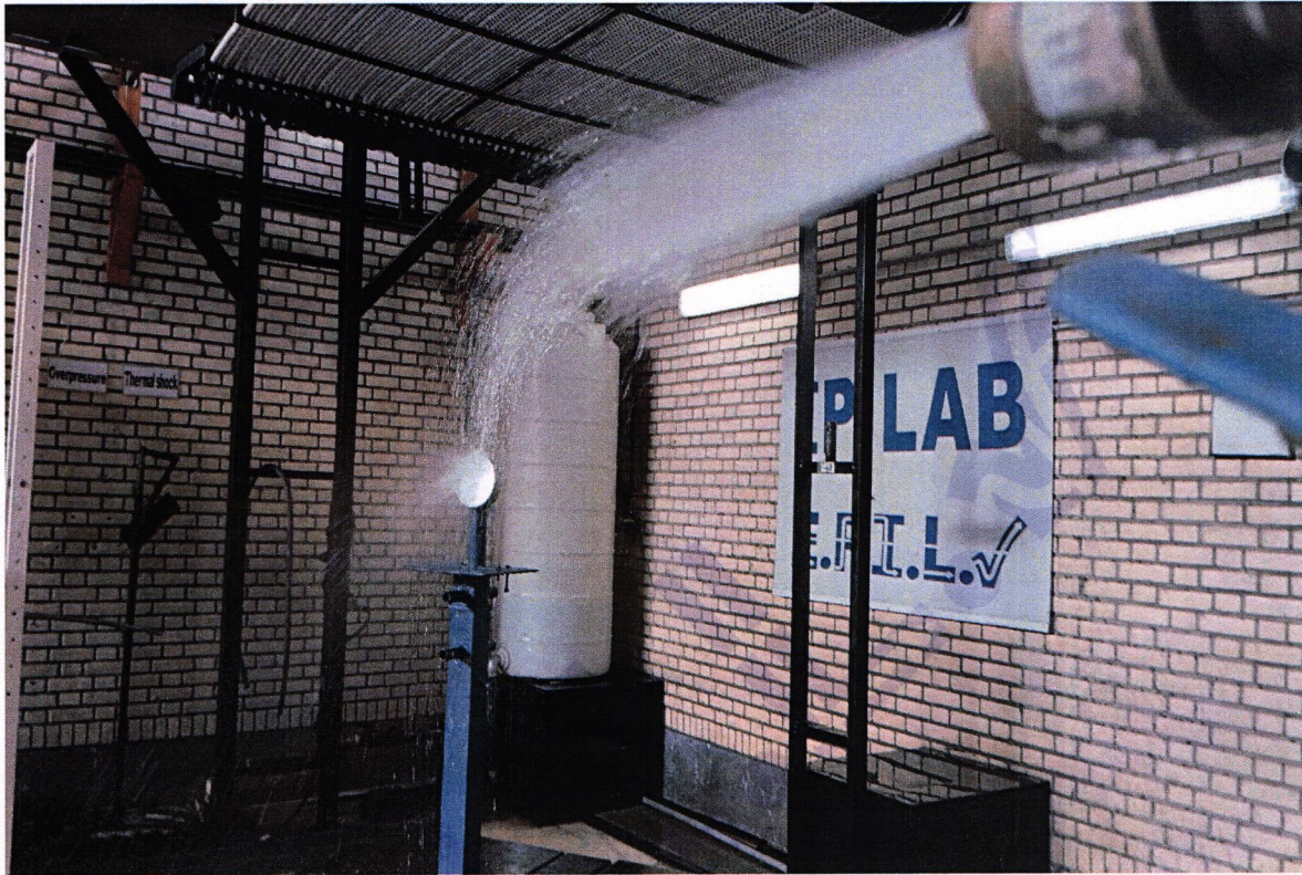
Figure 3: EUT under IPX6
